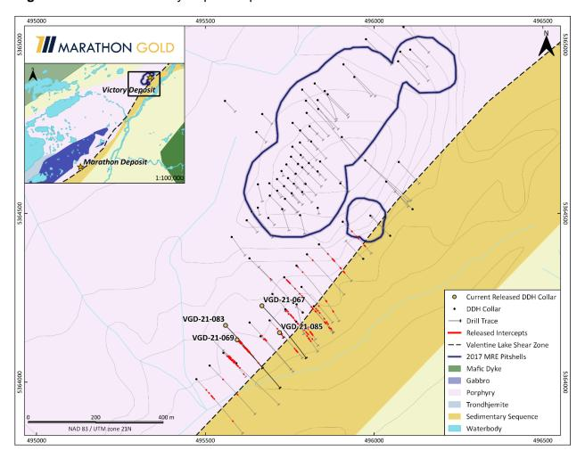
**Figure 5:** Long Section of the Victory Deposit (View NW) Incorporating all Drilling up to VGD-21-085, Representing 19,050 metres, and Assays Above 0.3 g/t Au (top) and 0.1 g/t Au (bottom).
