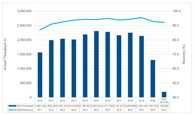
Figure 17-1: Processing Plant Throughput and Recovery
