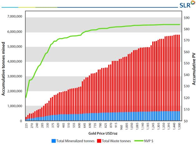
Figure 16-4: Pavón Central Pit Optimization – Pit by Pit Graph
