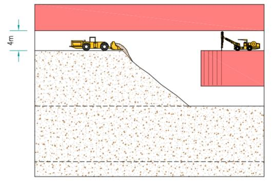
Figure 16-17: Avoca Method – Gap Left between Rock Pile and Bench
