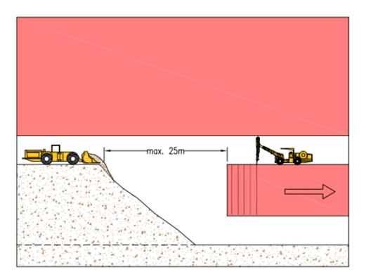
Figure 16-15: Avoca Method – Backfilling
