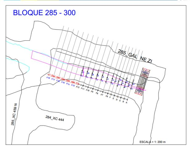
Figure 16-13: Avoca Typical Drilling layout - Plan
