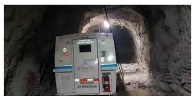
Figure 16-20: Portable Mine-Rescue Refuge Station at Jabalí West UG
