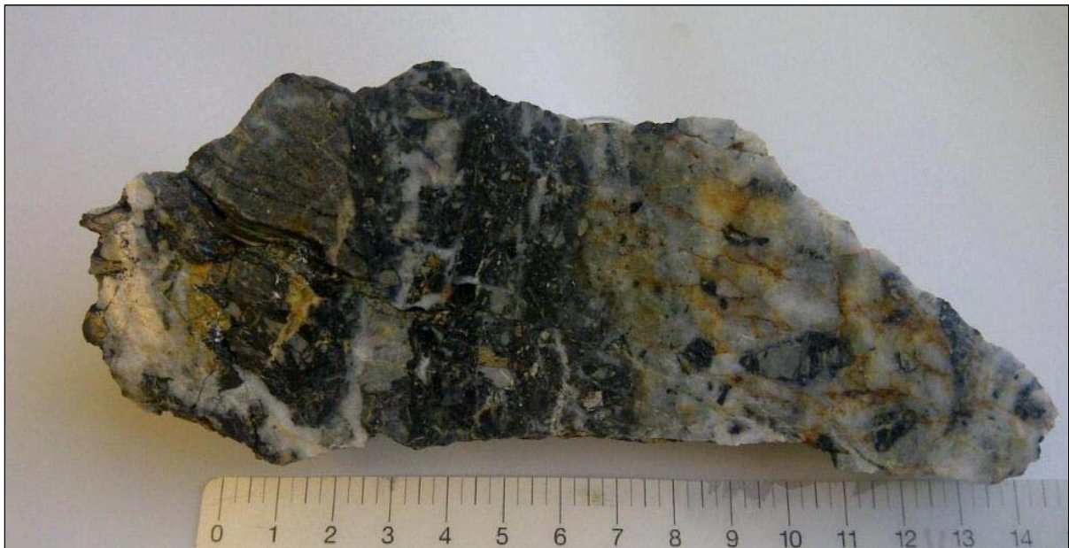
Figure 7.6 Gold bearing Quartz Vein from the Waste Dump of the Bonanza Mine
